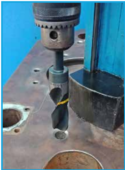
Install the fixture and drill the hole larger. Be careful not to drill too deep.
