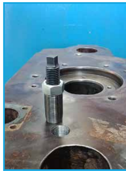
Screw the insert onto the installation tool and lightly coat the thread with thread locker. Screw the insert in the newly tapped hole.
