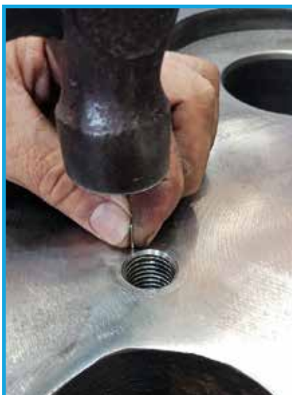
Install the locking pin to prevent the insert from ever rotating.
