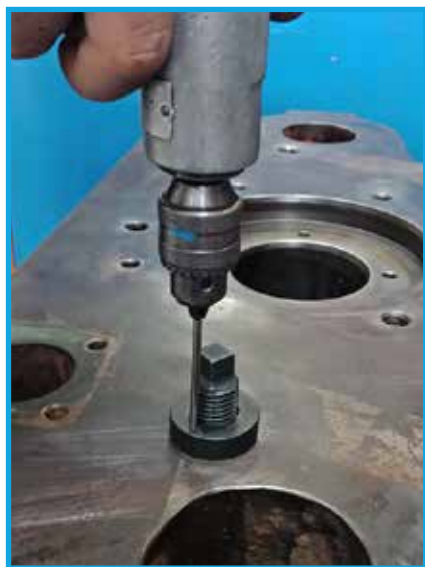
Using the fixture and drill provided, drill a small hole to accommodate the locking pin.
