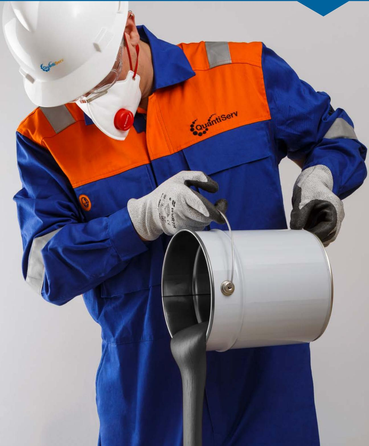
Epoxy resins can be used in a wide range of industrial applications, both indoors and outdoors. The industrial applications QuantiServ has worked on most frequently are the fixation of crane rails and equipment or skid foundations. We also have experience in the petrochemical industry on compressor grouting.
