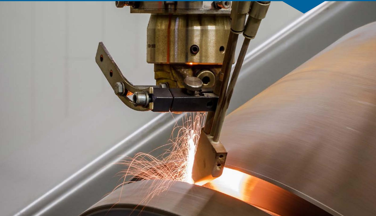
The introduction of robotized welding technologies has opened a new chapter in the reconditioning of marine spare parts. The latest innovation offers a vast range of advantages for the servicing of low-speed two-stroke piston heads.
